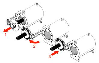
Figure 27: Burner Door Opening
