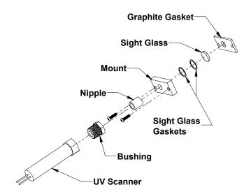
Figure 26: UV Scanner Assembly
