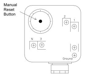
Figure 19: High/Low Gas Pressure Switch
