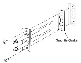
Figure 24: Igniter Electrode Assembly
