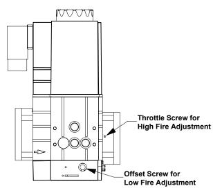
Figure 23: Gas Valve Air-to-Fuel Adjustment
