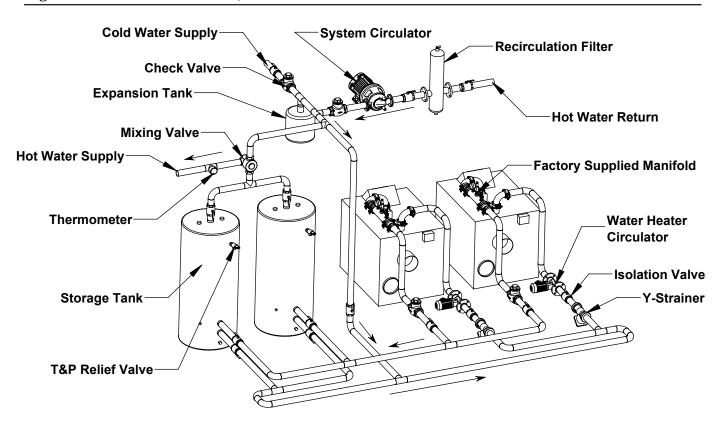
Figure 17: Two Water Heaters, Two Tanks
