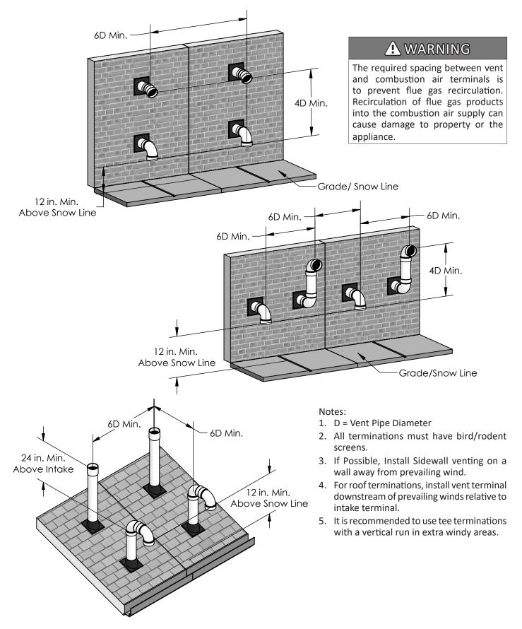
Figure 9: Multiple Appliance Direct Vent Termination
