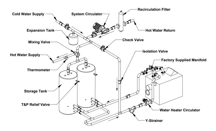
Figure 15: Single Water Heater, Two Tanks
