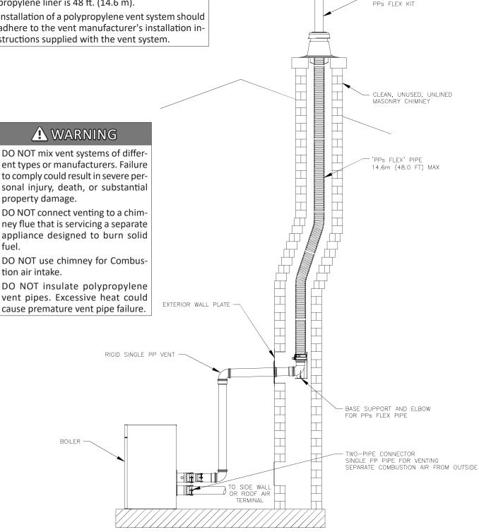
Flexible Vent in Masonry Chimney with Separate Combustion Air Intake Figure 10:
